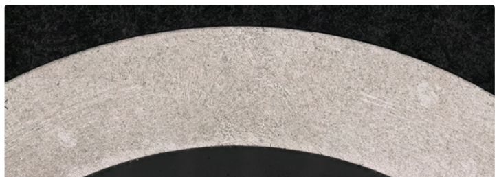
Figure 4: Cross Section After Drawing Tube Over a Mandrel
