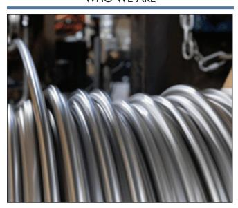
Specializing in welded and drawn 17-7 precision stainless steel tubing, we manufacture to spec – providing you with the lengths or special custom-fabricated forms for your medical device project. Our manufacturing facility is equipped to manufacture centerless ground tubing to +/-.00025" outside diameters.
