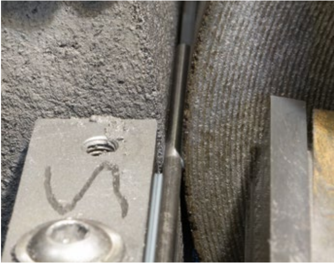
Figure 1: Centerless grinding enables OD tolerances as tight as +/- .00025"
